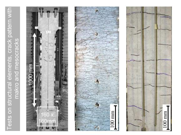
Interaction with the reinforcement leads to a complex multicracking with meso- and makrocracks.
